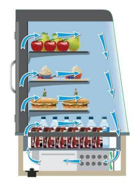
The food is cooled by a precisely controlled air flow pattern that maintains 38°F to 40°F within the cabinet, even though the customer side is open for self service.
